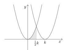
Since the graphs are symmetrical, we find the area shaded above, and double it. Again by symmetry, the curves intersect at  $x = \frac{1}{2}k$ :
